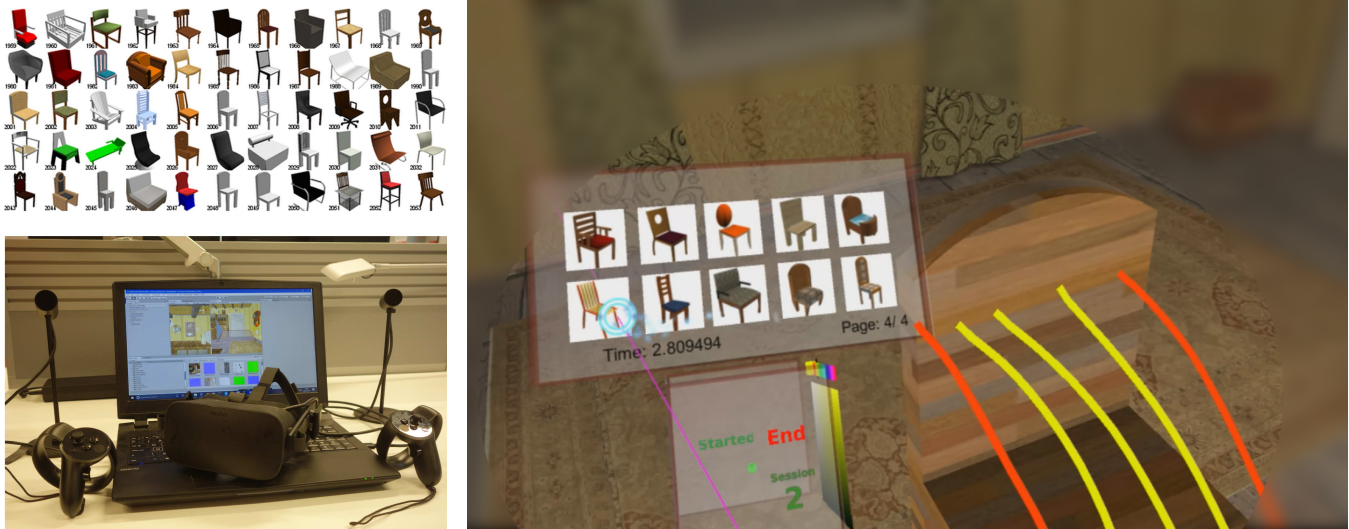
Figure 1: Our approach searches a dataset of chair 3D models (top left) using free-hand drawn sketches within a virtual reality. Our setup consists of Oculus RIFT, Oculus Touch and a laptop (bottom left). Sketches can be made either on top of a template chair or a prior search result (right).
