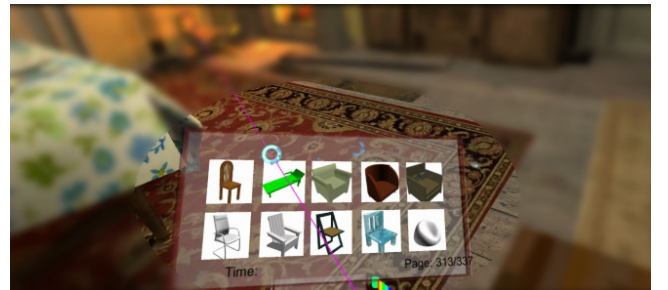
Figure 5: The scroll method provides a simple scrolling panel for navigating the database of all the chairs.
