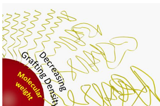
Figure 3.19. The grafting density (chain/nm 2 ) decreases with increasing molecular weight/chain length of the corresponding polymer (Benoit et al. , 2012).
