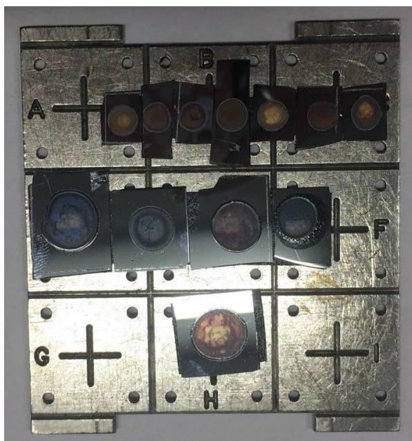
Figure 3.9. Sample preparation for XPS. The silicon wafer was cut to the desired size and used as substrate for drop-casting the colloids.
