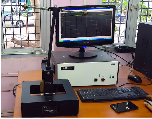
Fig. 2: Laboratory setup of pendulum system, ECP-Model 505.
