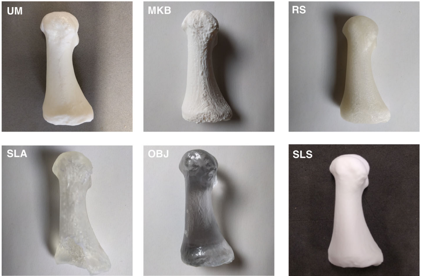
FIG. 3—Lateral views of six 3D printed replica metatarsals.
