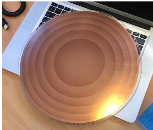
Figure 2. The completed 300mm metal mesh Fresnel lens.
