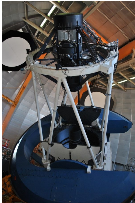
Figure 1 The Dark Energy Camera is mounted at the prime focus of the Blanco 4m telescope at CTIO. The covers for the primary mirror are open. The camera assembly, including the support cage, is approximately 3.6 m long and is secured to the inner telescope ring. The camera, not including the support cage and counterweights, weighs approximately 4350 kg. Subsequent to the date of this photo, the cage was retrofitted with aluminum side-covers. The aluminum covers of two of the four readout electronics crates are visible near the top of the camera, just underneath the “Top Cap”.
