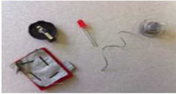
Figure 1. Flexible switch, battery holder, LED and conductive thread were used for the LilyPad Freestyle activity. (Photo by Anne Weibert)
