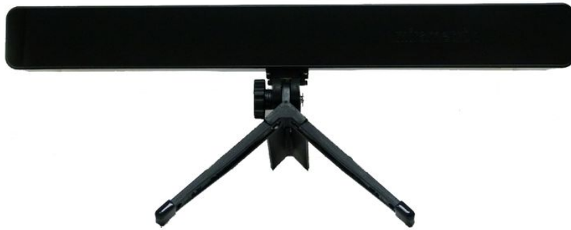
Figure 1. Mirametrix S2 eye-tracker and tripod. The rectangular device is the eye tracker, and the tripod (3 legs) is the device used to hold the eye tracker in place. The eye tracker is equipped with two cameras located on the right and left corners, and an infrared light located in the middle hidden within the device. The eye tracker was situated under the screen and slightly moved to best fit to the participant's eyes. The S2 Mirametrix eye tracker can view the participant's eye from a distance.
