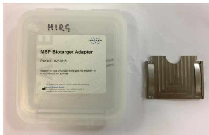
Figure 5-1: A Biotarget adapter was required to fit in the Biotarget plate into the MALDI-TOF Microflex instrument.
