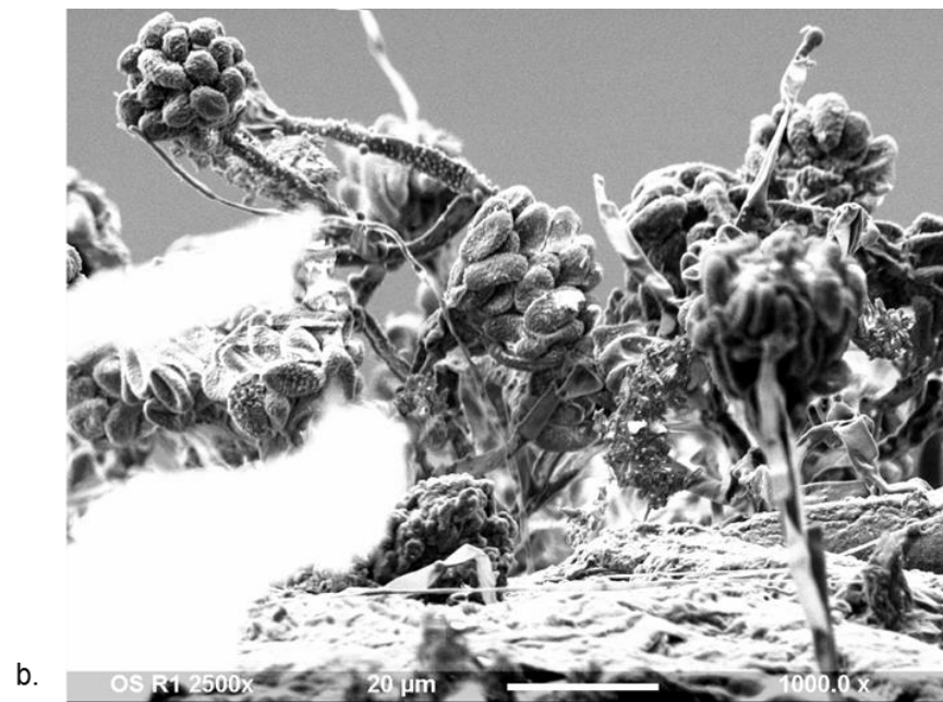
Figure 7-35: Fungal growth on gypsum board following pre-inoculation OS treatment at 2500 ppm. a. Surface; b. Cross-section using SEM images at 1000x magnification. The arrows marked in red indicate fungal growth from within the porous area and yellow indicates flat exposed surface with no growth.
