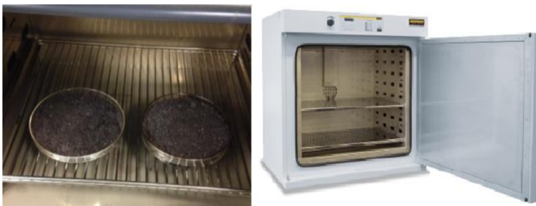
Figure 3.2: (a) SCG samples contained in pyrex petri dishes during drying, (b) Exterior of oven model used in drying experiments (adapted from “ http://www.keison.co.uk/nabertherm_tr.shtml ”).
