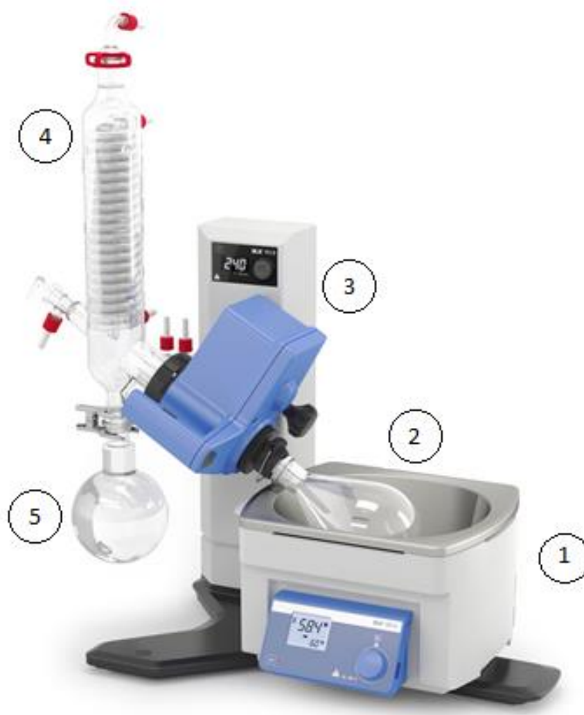
Figure 3.10: Rotary evaporator key operating features (adapted from “ http://www.ika.com/owa/ika/catalog.product_detail?iProduct=10002170 ”).
