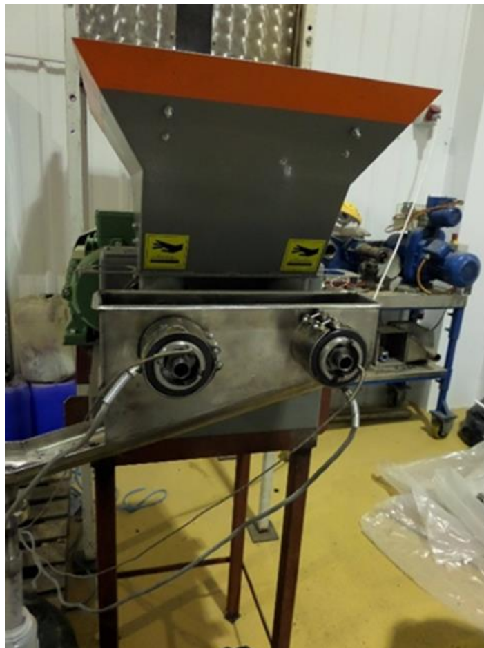
Figure 3.14: Screw press used for SCG mechanical expression.
