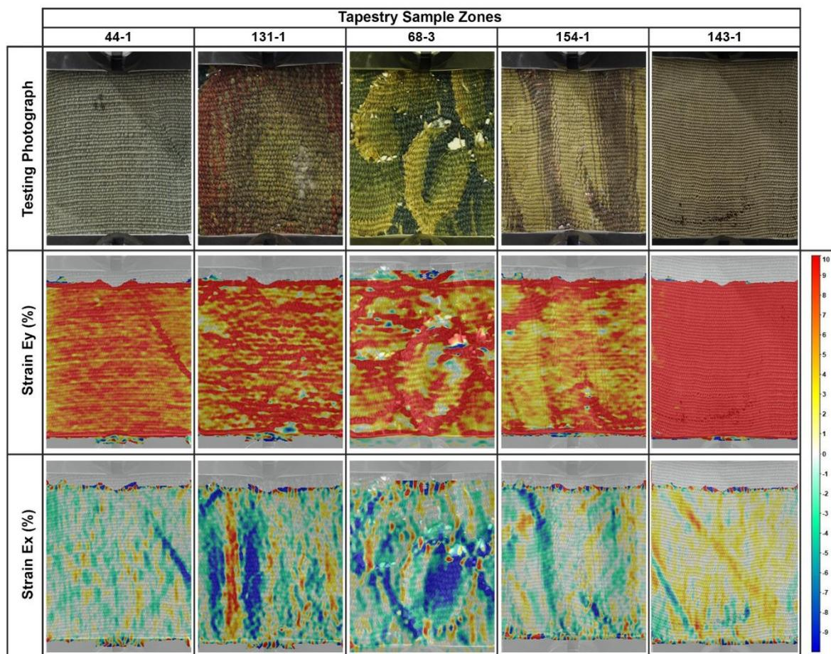
**Figure 3.** DIC results for vertical and horizontal strain distribution in 5 tested samples.
