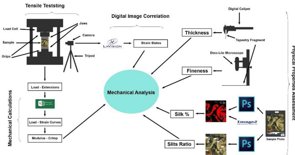
**Figure 1.** Methodology used to characterize and test the samples.
