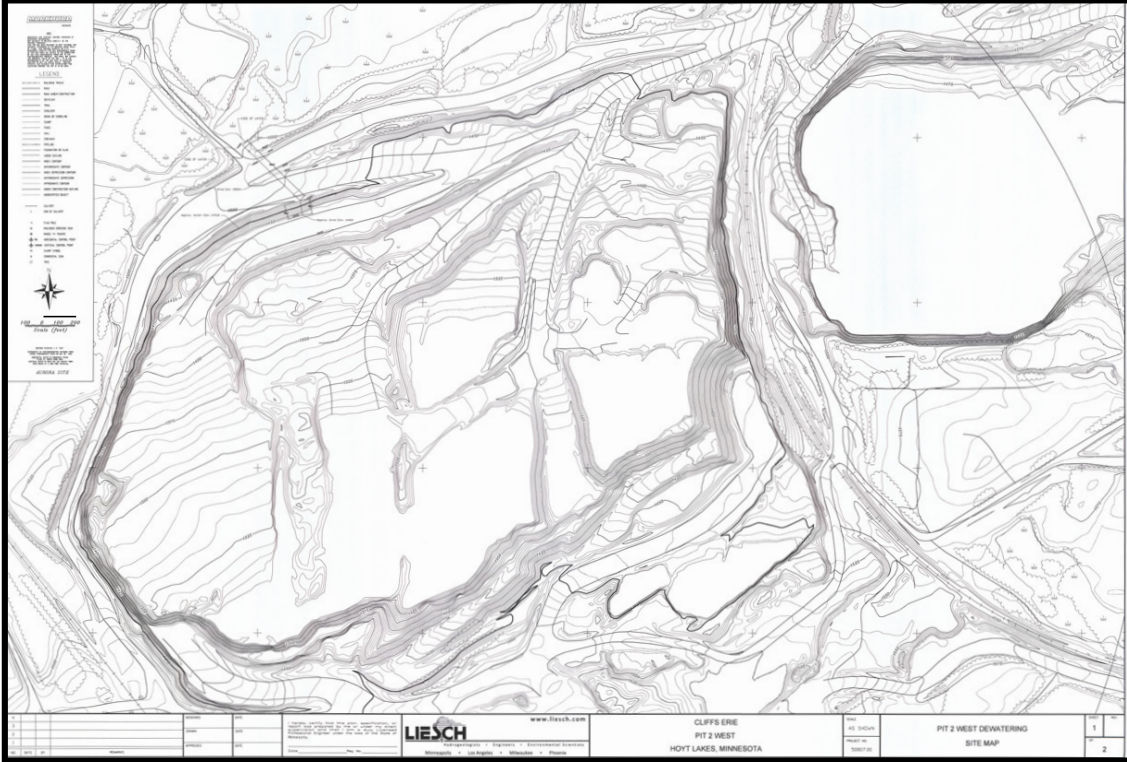
Figure 2.6: Topographic map of the Wentworth Pit 2W, based on a survey conducted when it was just starting to fill up with water. The areas in the lower centre of the pit are the deepest, with at least 50 m depth. Image taken from Ref. [93].
