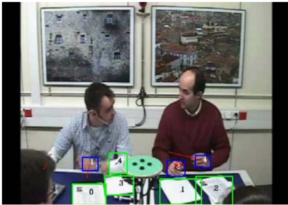
Fig. 2. Hands and paper tracking. Red lines show the trajectory of each hand. The red line on the lower left denotes a hand that is currently occluded but that has been tracked in previous frames. Fig. 3. Tracking of hand #1 over selected meeting epoch. Displacement of hand in each successive frame (pixels) from automatic tracking (AUTO) and manual annotation (Ground Truth GT).
