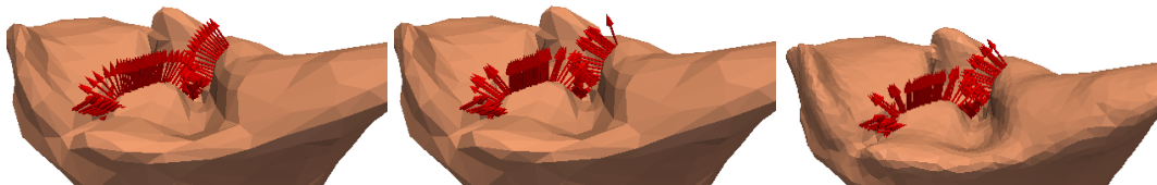
Figure 5. Left: C0 normals (red arrows) on a low-resolution liver mesh. Centre: Constant normals on low-resolution mesh. Right: Constant normals on high-resolution mesh.
