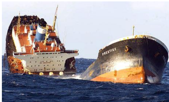
Fig. 1: The prestige oil tanker incident in 2002 is an example of hull girder collapse ( https://globalvoicesonline.org/ ).
