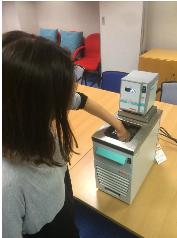
Figure 9: The Julabo F-12 Refrigerated Circulator used for the cold pressor task. This equipment was chosen for the experiment as it had a temperature resolution of 0.01°C and provided constant water circulation.
