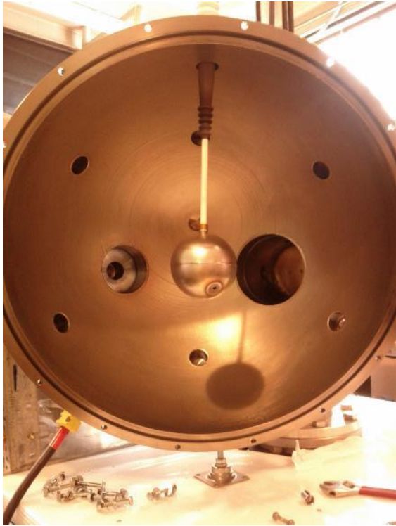
Figure 6. Photograph of the spherical plasma probe mounted in place of the cathode grid. The small black spot on the bottom is a hole drilled to eliminate virtual leaks from the probe.
