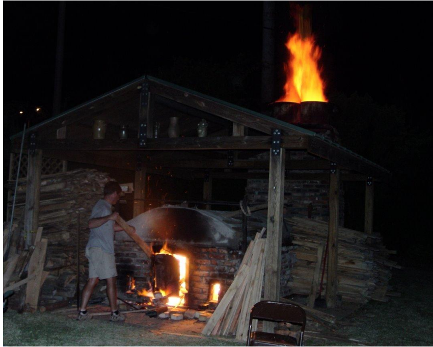
Figure 6.2. Contemporary groundhog kiln with wooden superstructure, Aiken, South Carolina. Courtesy Gary Dexter.
