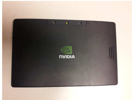
Figure 3.1: NVIDIA developer tablet with Tegra 3 processor and stereo cameras.
