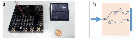
Fig. 2: a) A matrix array of photodiodes and a large-surface detector measuring approximately 5 x 5 cm and b) Multipath effect on light entering and exiting a phantom onto a large detector.
