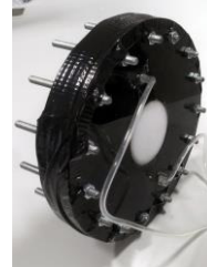
Fig. 1: Liquid tissue phantom: an acrylic container through which a scattering liquid (milk, Intralipid) mixed with a dye is recirculated. A diffusive window allows coupling of light into the phantom
