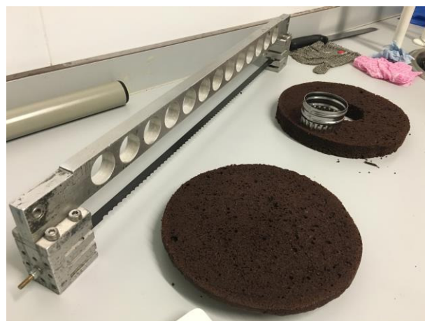
Fig. 1. Use of sponge cutting fixture and 3 cm circular stencil to prepare a chocolate sponge.
