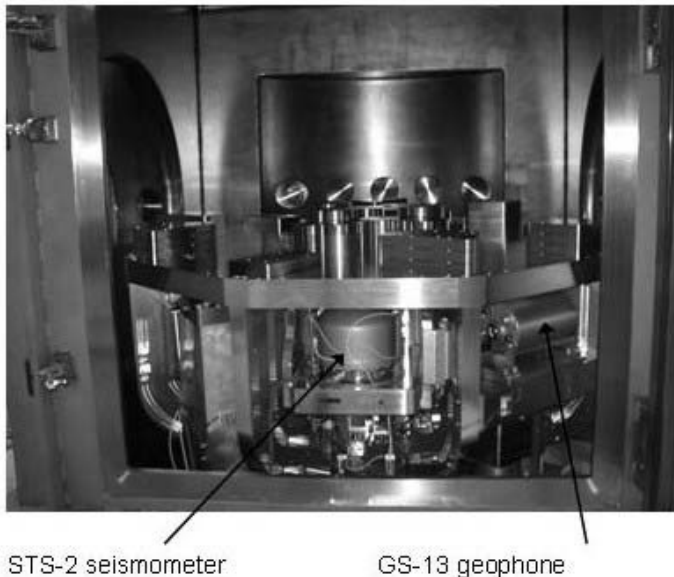
Figure 5. Picture of the Advanced LIGO seismic isolation technology demonstrator two-stage active platform inside the vacuum tank. The two stages are structurally interleaved to correctly position the centers of gravity. One of the 3 STS-2 seismometers mounted on the first stage, and one of the Geotech GS-13 geophones mounted on stage two are indicated. The overall width is approximately 1.5 m. Masses simulating the load of the suspension system can be seen on the optics table which is part of stage two of the platform.
