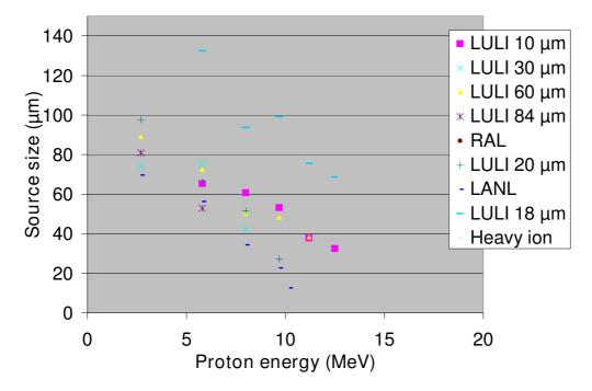
It's remarkable, that the  $d_{max}$  doesn't depend significantly on the target thickness but on the laser intenstiy.
