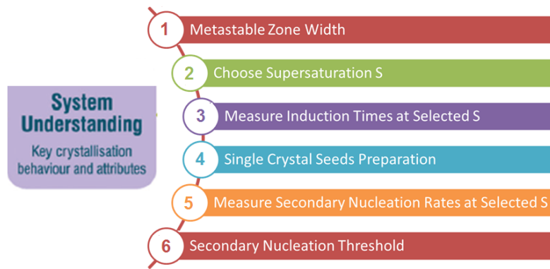
Figure 12: Workflow for secondary nucleation, which allows system understanding. Stage 1: The solubility and the MSZW are the starting points to identify the conditions to crystallize the material at the selected concentration and temperature. Stage 2: The supersaturation ratios for secondary nucleation studies are selected within the MSZW. Stage 3: Induction time experiments at the selected supersaturation ratios are required in order to determine the time frame for seeding experiments avoiding unwanted primary nucleation. Stage 4: The crystals that will be used as seeds need to be well-characterized. Stage 5: The conditions for the secondary nucleation experiments are established and now the seeded crystals can be added and secondary nucleation can be monitored at the selected conditions of supersaturation. Stage 6: Analyzing the secondary nucleation rates at different supersaturated conditions in order to determine the secondary nucleation threshold S_d understanding at which supersaturation ratio secondary nucleation is negligible.
