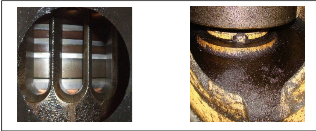
Figure 17. The piston rings and the bottom of scavenging box when using the new system
