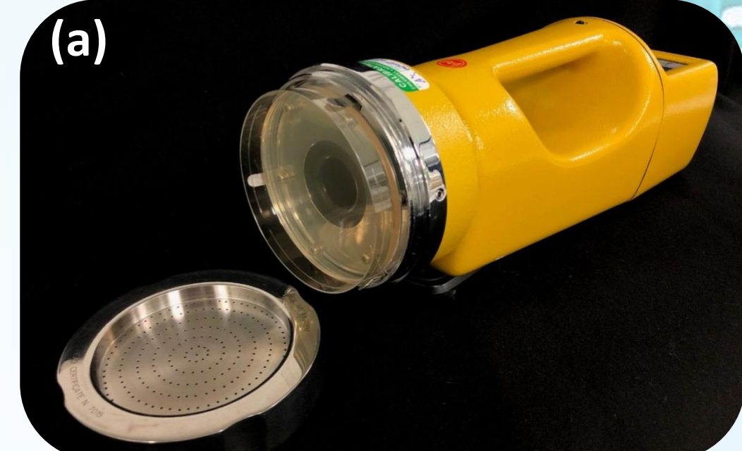
Fig 1. (a) SAS Super 180 Air Sampler with fitted TSA plate and separate aspirating head and (b) ICU patient isolation room layout showing position of air sampler.
