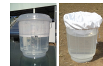
Figure 9: Two prototype systems to be field tested over 12 months (2018 – 2019) (1) SODIS bucket with cloth pre-filter
