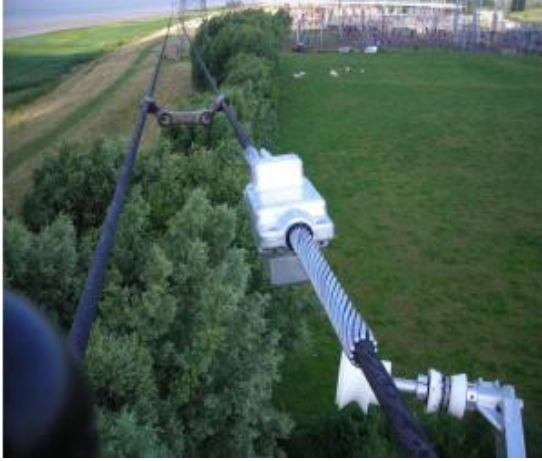
Fig. 2-20. Ampacimon smart sensor [64]
