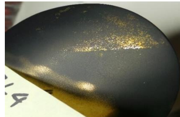
Figure 10 Experimental cavitation erosion tests by Mantzaris et al., (2015).
