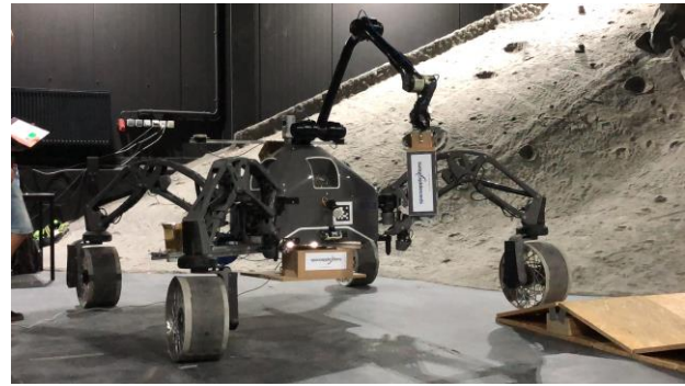
Fig. 15. SherpaTT during its movement on uneven terrain (wooden obstacle) with the primary APM (below) and the auxiliary APM (docked on the manipulator) (credit: DFKI GmbH)
