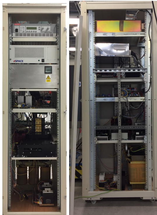
Figure 3.1: Pictures of the 10 kVA inverter with customizable control strategy (front and side view).
