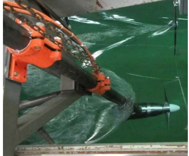
Figure 1. Turbine installed at the tow tank at CNR-INSEAN
