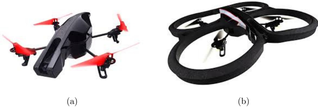
Figure 3: AR.Drone 2.0 configurations for (a) Outdoor navigation (light configuration) and (b) Indoor navigation (protected by external hull).
