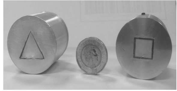
Fig. 13. SG fractal (left) and conventional composite (right) ultrasonic transducer.
