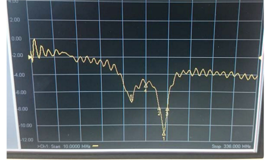
Fig. 3 Frequency response of the antenna
