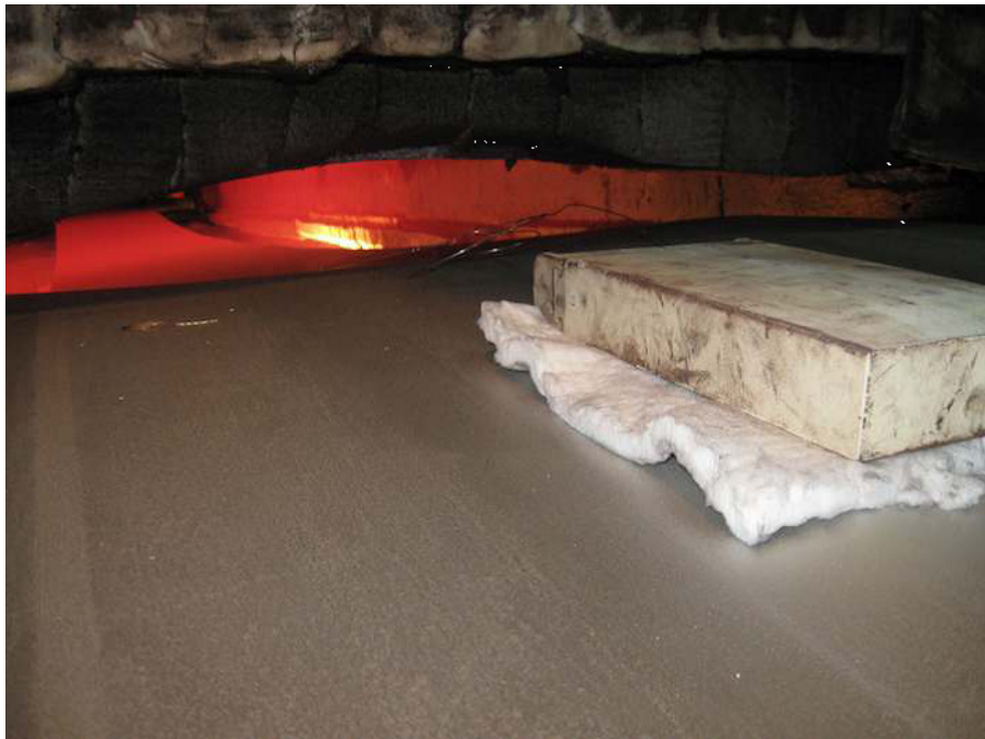
Figure 3.63: Test with one thermocouple connected to the DataPaq, going into the furnace
