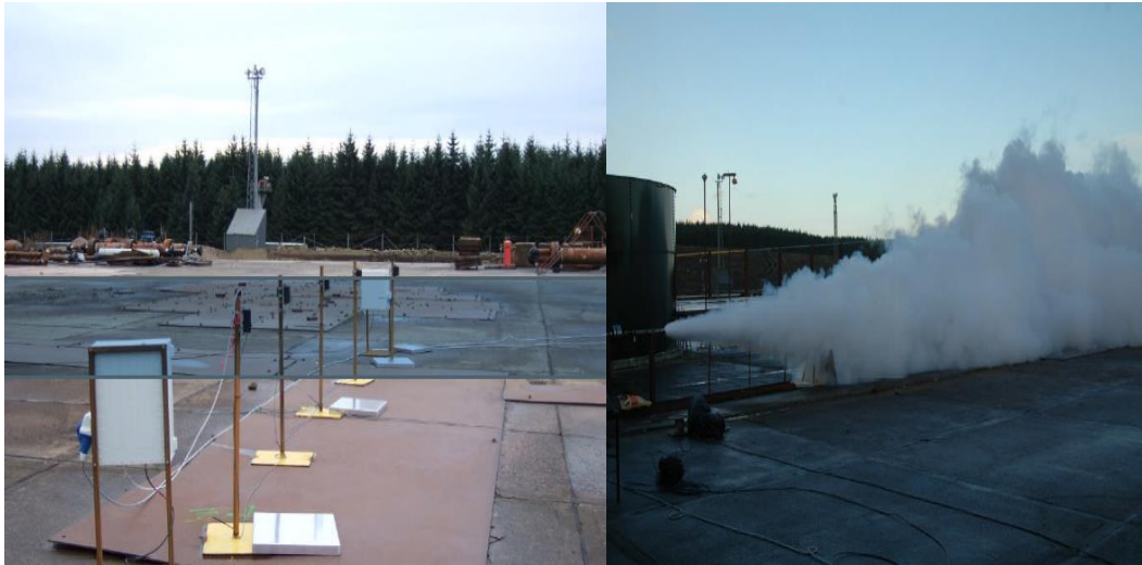
Figure 14. Photographs of the instrumented target and of a release of CO 2 through a 0.5 inch orifice [142]
