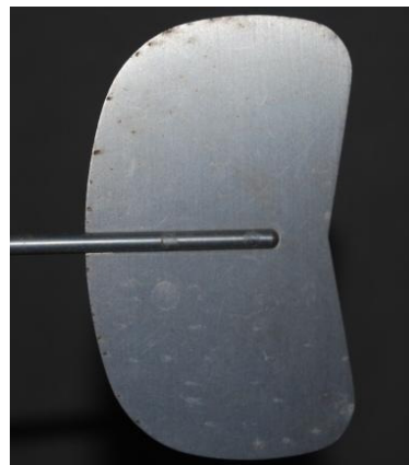
Figure 3: Wind vane following suspected lightning strike
