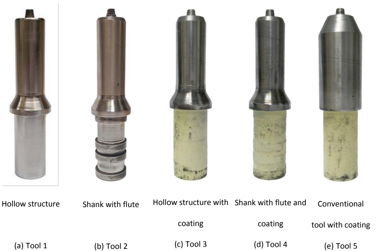
Figure 2. Fabricated FSW tools with heat insulation features [20].
