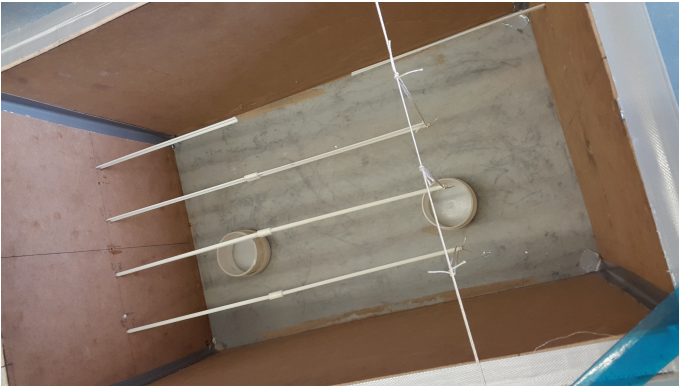
Figure 3: Box prior to pluviation
