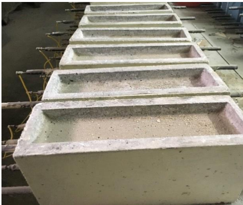
Figure 3. Epoxy coated specimens following ASTM G 109-2005 (drying and wetting cycles)
