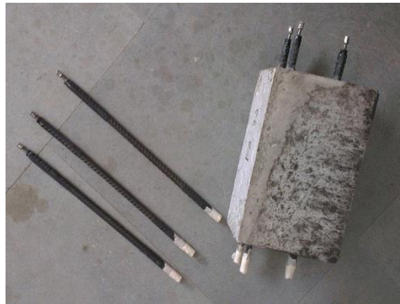
Figure 2. Steel bars and concrete specimen (ASTM G 109-2005)
