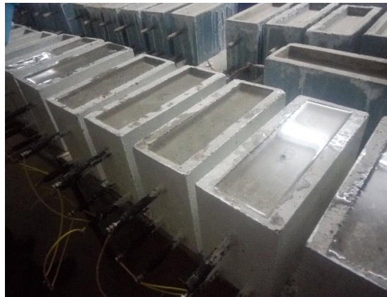
Figure 3. Epoxy coated specimens following ASTM G 109-2005 (drying and wetting cycles)
