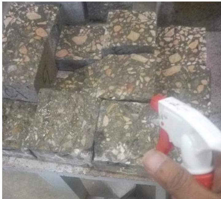
Figure 7. Spraying of 0.1 N silver nitrate solution on freshly split concrete specimens
