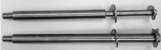
Figure 2. Photograph of optimized (upper) and standard uniform (lower) screw piles tested in the centrifuge.
