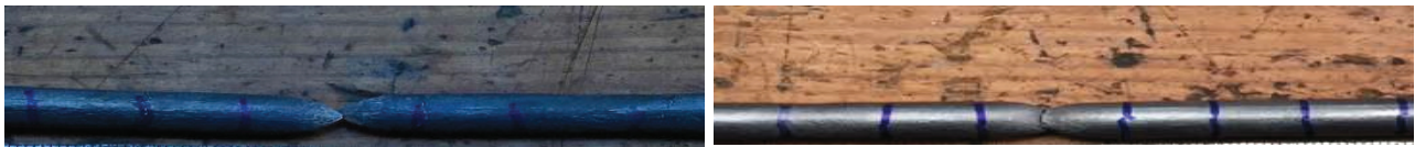
(a) Fracture of Pb
