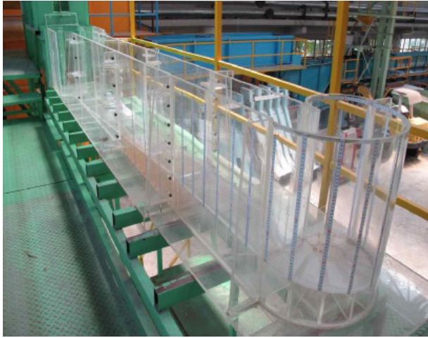
(a) Approach channel with the high-elevation tank
