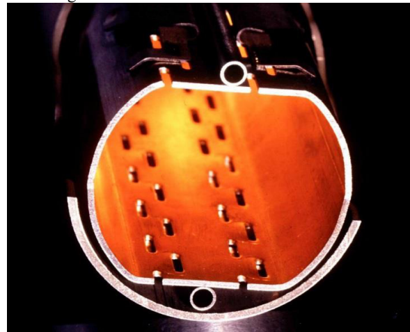
Figure 1: The LHC beam screen.
