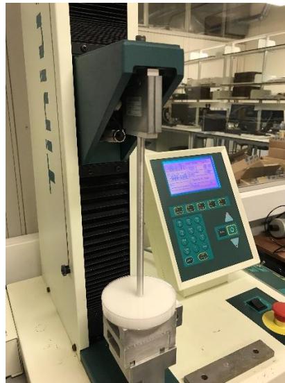
Figure 4. Setup for spherical indenter, ramp-hold relaxation test. It was implemented on a Tinius Olsen H5KS material test machine with an 8 mm diameter spherical-tipped aluminium indenter.
