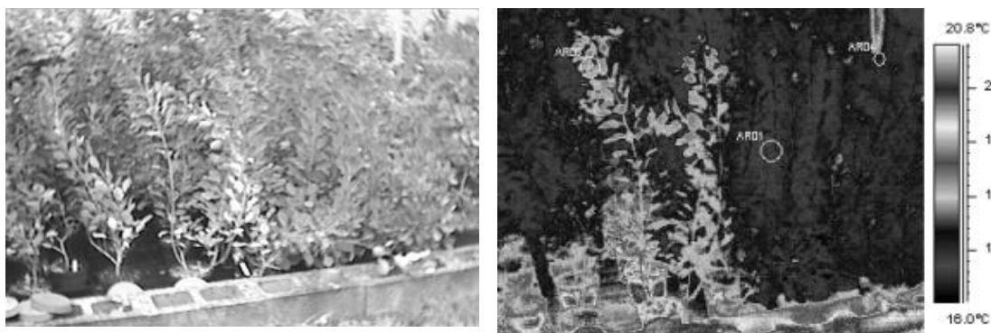
150 Figure 1. The left-hand panel shows a visible (RGB) image of some potted Cotinus plants, while the right-hand panel shows the corresponding thermal image obtained using a hand-held thermal camera (FLIR SC2000). This example illustrates the utility of thermal sensing as
