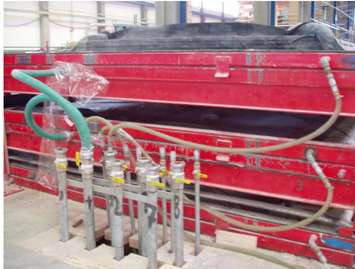
Figure 1. Manufacturing of cross-laminated timber panels: vacuum press.
