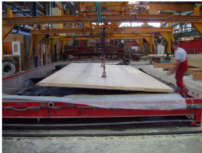
Figure 2. Manufacturing of cross-laminated timber panels: removing the resulting panel from the press.
