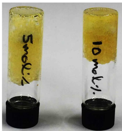
Figure S4.56. Photograph of the reaction mixtures of \text{Ph}(\text{CH}_2)_2\text{NH}_2 \cdot \text{BH}_3 with the crosslinker \text{BH}_3 \cdot \text{NH}_2(\text{CH}_2)_8\text{NH}_2 \cdot \text{BH}_3 in different ratios (left) 5 mol % cross-linker and (right) 10 mol % crosslinker and 1 mol% of \text{IrH}_2(\text{POCOP}) in THF.
