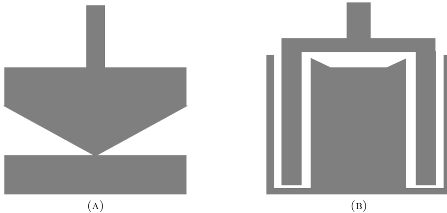
FIGURE 2.11: Cross sections of the two geometries used, a cone and plate geometry (A) and a double gap geometry (B).
